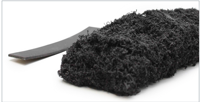
FLEXILOCICE before and after exposure to fire.
