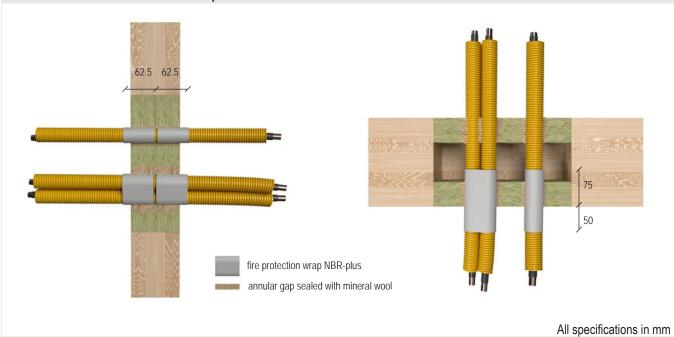
Wall **NBR-plus** Fire Outer Number of wraps [n] Overlap Inside seal Outside [mm] [mm] seal [mm] [n] Wrap width Service diameter resistance [mm] class [mm] **Electrical installation conduits** made of plastic, single, ≤ 32 1 with/without cables  $\leq$  21 mm 47.5-50.0 12.5-15.0 62.5 2 EI 90 U/U ≤ 32, **Electrical installation conduits** made of plastic, bundled, bundled to 2 with/without cables  $\leq$  21 mm ≤ 100
