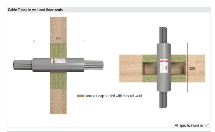
Wall Services Fire resistance class Outer diameter [mm] Cables ≤ 21 EI 90 Cable bundles ≤ 100 Floor Services Fire resistance class Outer diameter [mm] Cables ≤ 21 EI 90 Cable bundles ≤ 100
